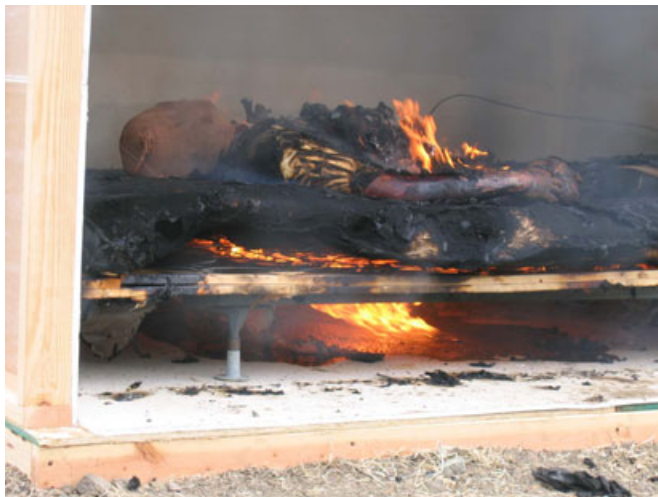
FIG. 8—Test 2: at 1 h 40 min: the blanket and clothing were largely consumed, but the fire was visible involving the lower torso and pelvic area. Note that the nylon stocking over the head is unburned. Pool of rendered fat beneath the box spring is beginning to ignite. Photograph by John DeHaan.
