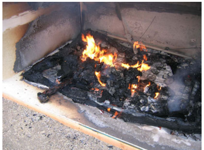
FIG. 9—Fire at 5 h 14 min. Flames less than 12 inches (30 cm) above body in height. Photograph by John DeHaan.
