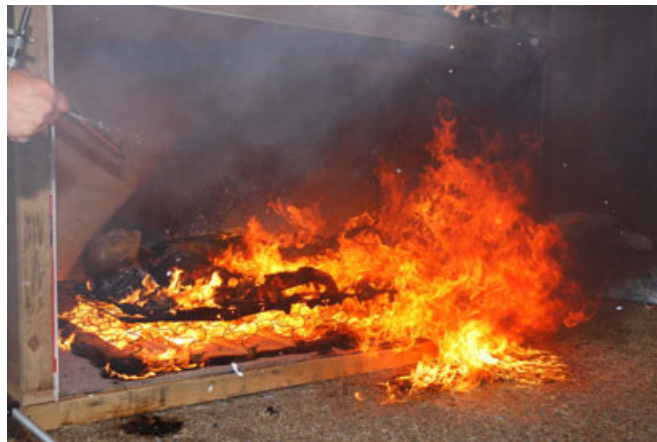
FIG. 1— Test 1: fire at 16 min: box spring and carpet fully involved, driving fire growth. Photograph by Jamie Novak.
