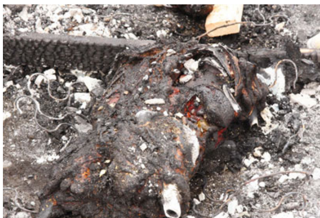
FIG. 13—Test 3: body after 11 min of postflashover exposure (15 min of total fire duration) is extensively charred on exterior, but torso and internal organs are still intact (femurs cut prior to test). Photograph by Jamie Novak.
