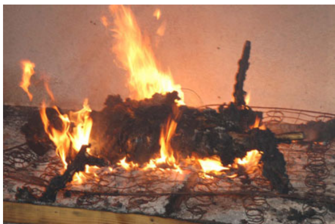
FIG. 4—Fire at 3 h 27 min. The metal springs are supporting the body (fuel source) above the flames where the charred carpet and wood floor are acting as a wick for the rendered body fat. Photograph by Elayne Pope.
